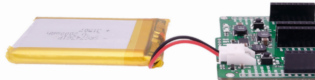
Figure 1-2: Connecting Li-Polymer battery
