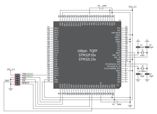
Figure 7-2: Connection schematics for 100-pin STM32F10x/ STM32L15x MCU via 2x5 male header
