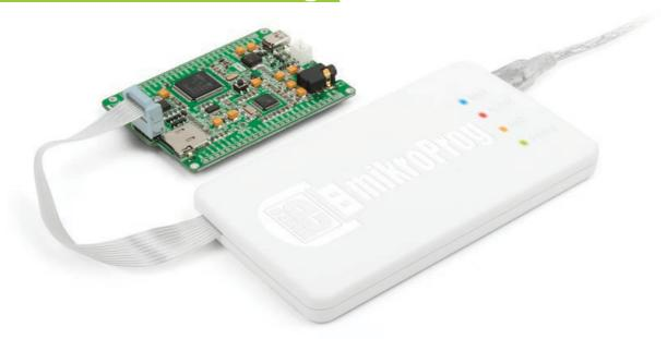
mikroProg<sup>™</sup> for STM32® is a fast programmer and hardware debugger. Smart engineering allows mikroProg<sup>™</sup> to support all STM32® ARM® Cortex<sup>™</sup>-M3 and Cortex<sup>™</sup>-M4 devices in a single programmer! Outstanding performance, easy operation, elegant design and low price are it's top features. It is supported in mikroElektronika, as well as in other ARM® compilers.
