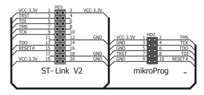
Figure 6-3: mikroProg<sup>™</sup> to ST-Link V2 adapter connection schematics
