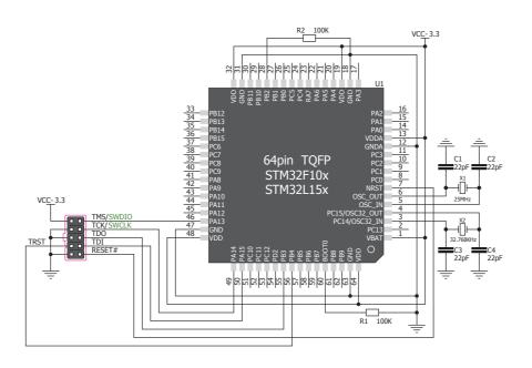
Figure 7-1: Connection schematics for 64-pin STM32F10x/STM32L15x MCU via 2x5 male header
