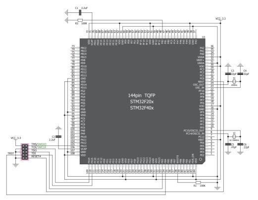
Figure 7-4: Connection schematics for 144-pin STM32F20x/STM32F40x MCU via 2x5 male header Page 20
