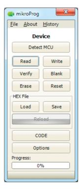
mikroProg<sup>™</sup> for STM32® programmer requires special programming software called mikroProg Suite<sup>™</sup> for ARM®. This software is used for programming all of STM32® ARM® Cortex<sup>™</sup>-M3 and Cortex<sup>™</sup>-M4 microcontroller families. It features intuitive interface and SingleClick<sup>™</sup> programming technology. Software installation is available on following link:
