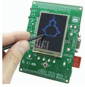
The board contains a 320x240 Touch Screen Panel, 4-way joystick, Microchip's MCP9700A Temperature Sensor, optional MRF24J40MA ZigBee Module, headphone and microphone connectors, RS-232 port, and prototyping pins.
