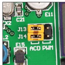
Figure 16-3: Jumpers J13 and J14 in ACD position
