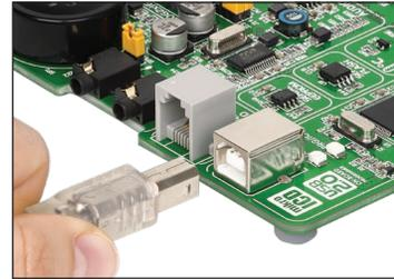
Figure 3-2: USB connector's front side
