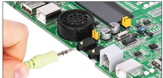
Figure 16-2: 3.5mm connectors CN22 and CN23
