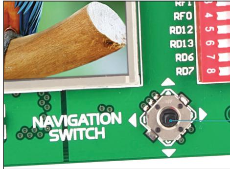
In addition to navigation function, the joystick can serve as a push button
