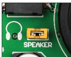
Figure 16-5: Enabling on-board speaker
