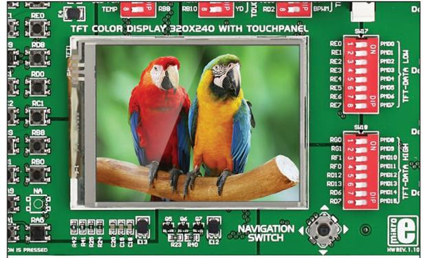
Figure 18-1: TFT display with touch panel
