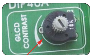
Figure 24 GLCD contrast adjustment potentiometer
