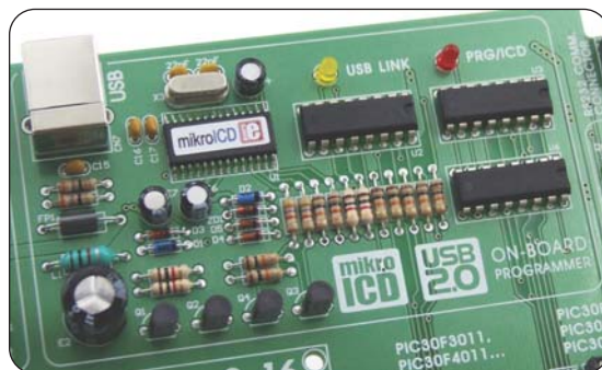
Figure 12 On-Board USB programmer with mikroICD
