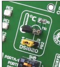
Figure 10-2: J9 en position gauche (communication 1-wire via PA4)
