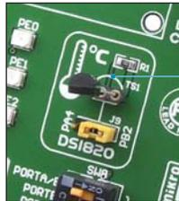
Figure 10-3: J9 en position droite (communication 1-wire via PB2)
