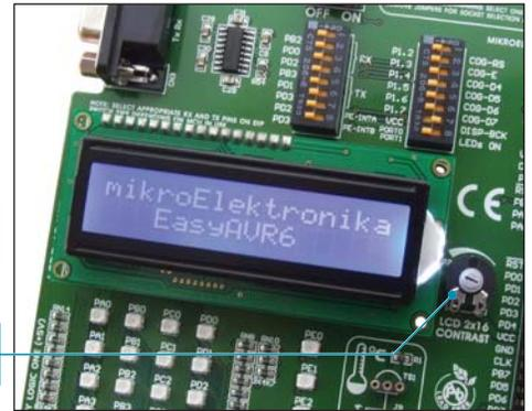
Figure 15-2: Afficheur LCD 2x16
