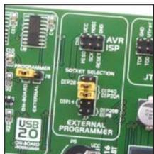
Figure 4-1: Placement du jumper J7
