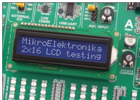
Figure 17-1: Alphanumeric LCD connector
