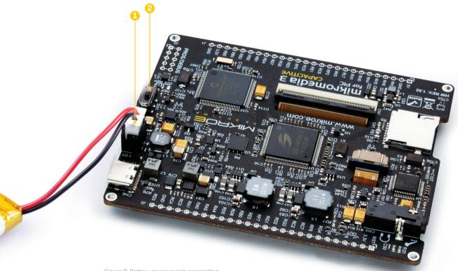
Figure 8: Battery power supply connection
