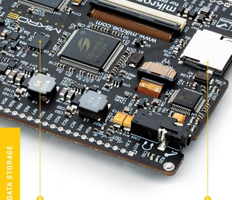
Figure 10: MicroSD card slot view
