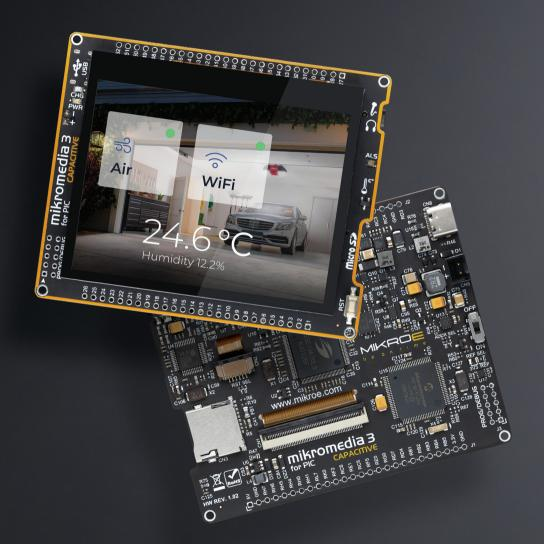
mikromedia 3 for PIC CAPACITIVE is a compact development board designed as a complete solution for the rapid development of multimedia and GUI-centric applications. By featuring a 3.5" capacitive touch screen driven by the powerful graphics controller that can display the 24-bit color palette (16.7 million colors), along with a DSP-powered embedded sound CODEC IC, represents a perfect solution for any type of multimedia application.
