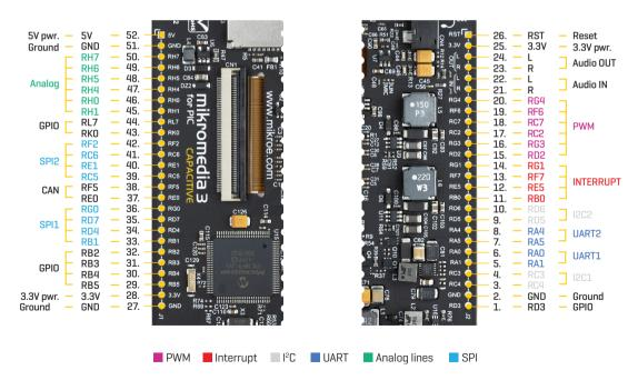
Figure 13: 1x26 pin header view
