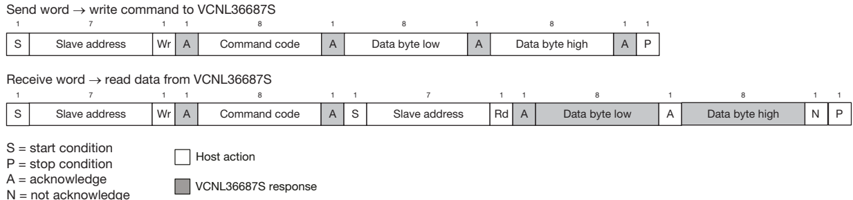
Fig. 9 - Write Word and Read Word Protocol
