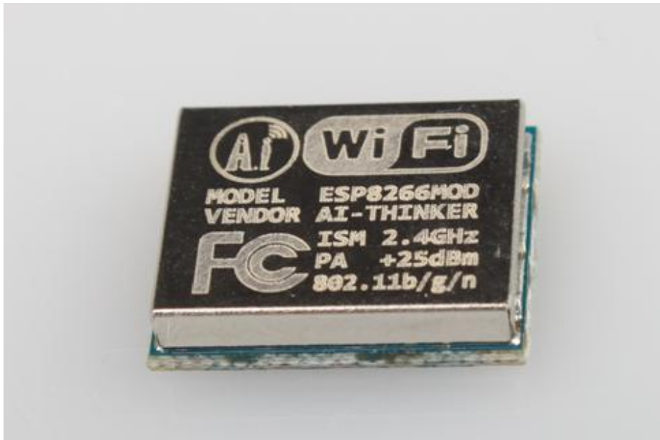
Figure 2 [Module Pin Counts, 20 pin, 16.2mm x 13.2mm x 3.0 mm]
