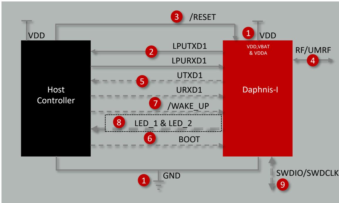
Figure 13: Minimal pin connections
