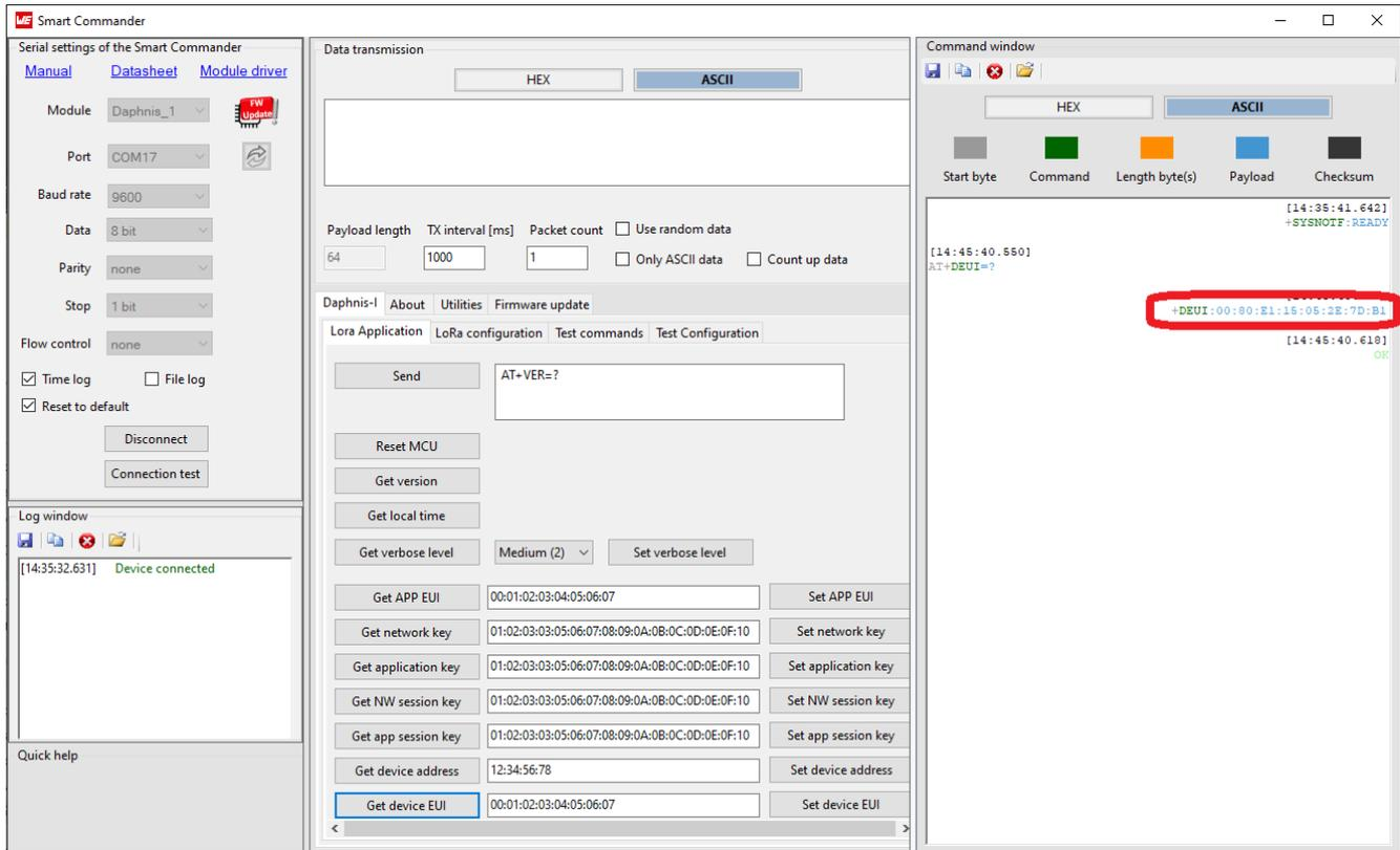
Figure 18: Smart Commander AT+DEUI command
