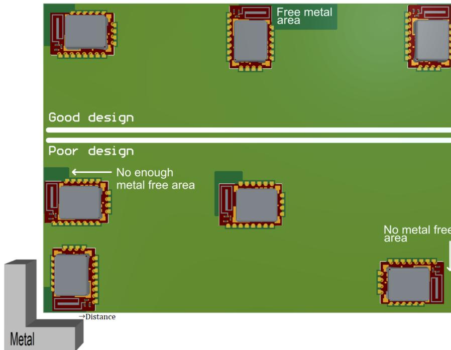
Figure 35: Placement of the module with integrated antenna
