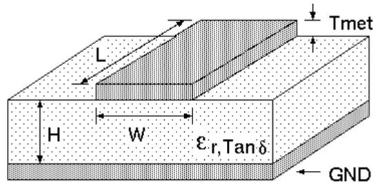
Figure 36: Dimensioning the antenna connection as micro strip
