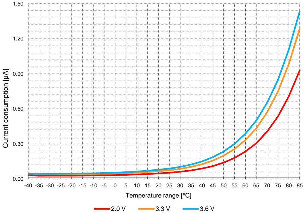
Figure 3: Current consumption during Sleep mode
