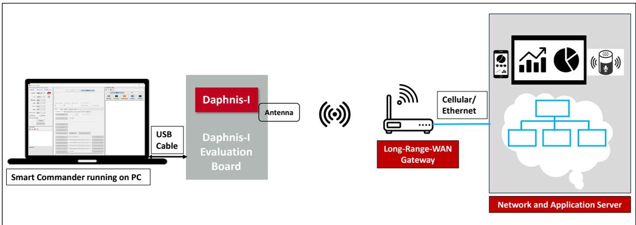
Figure 15: Daphnis-I quick start setup
