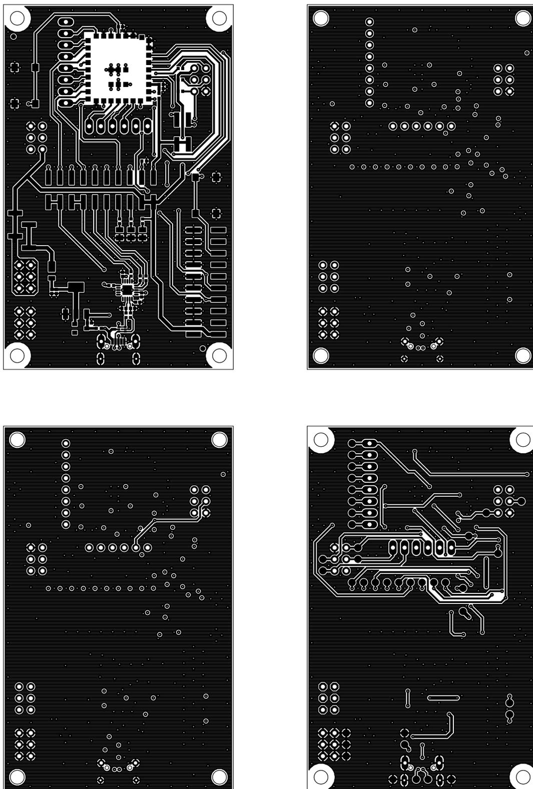
Figure 42: Top layer (upper left), second layer (upper right), third layer (bottom left), fourth layer (bottom right)
