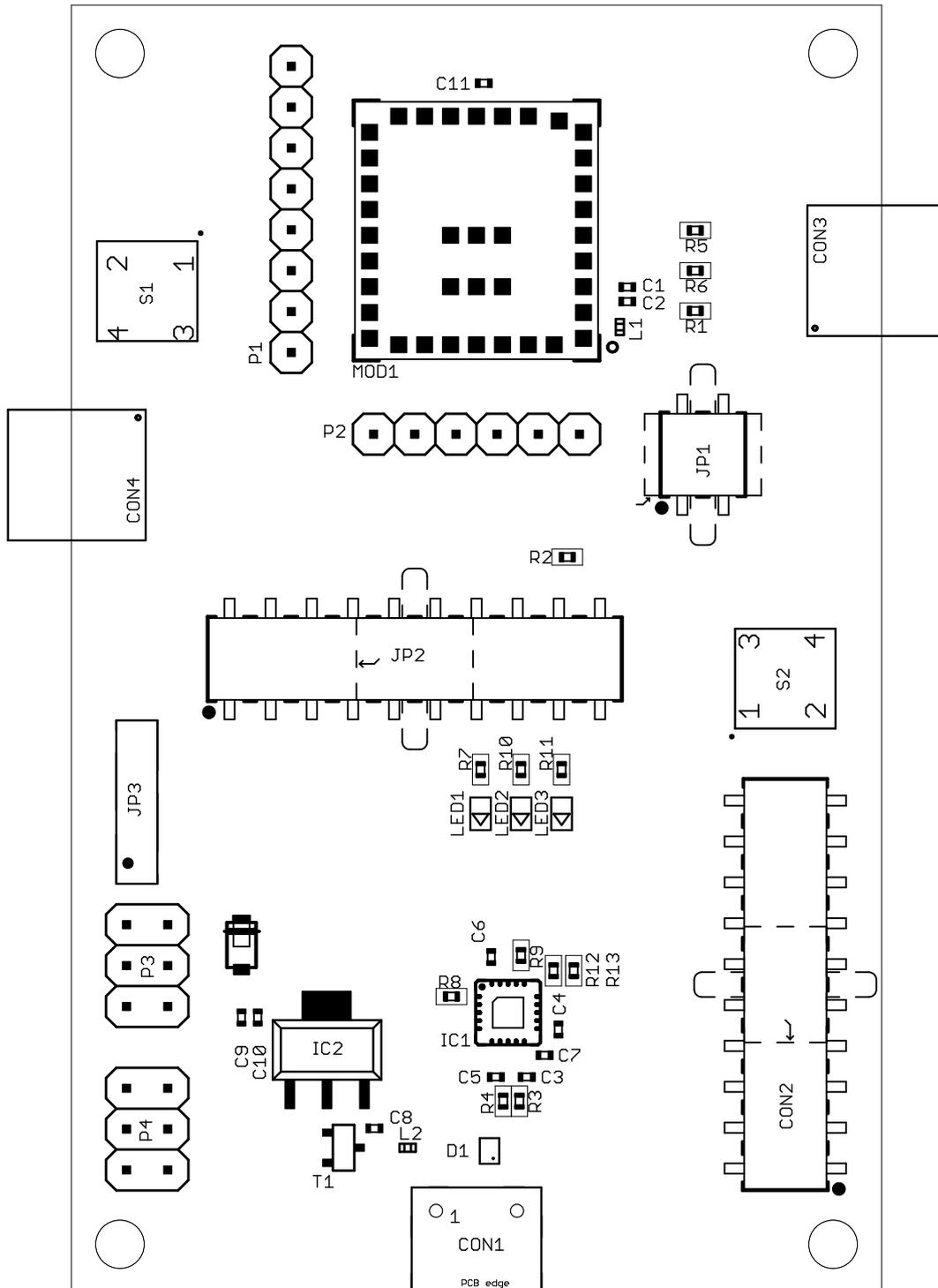
Figure 41: Reference design: Assembly diagram
