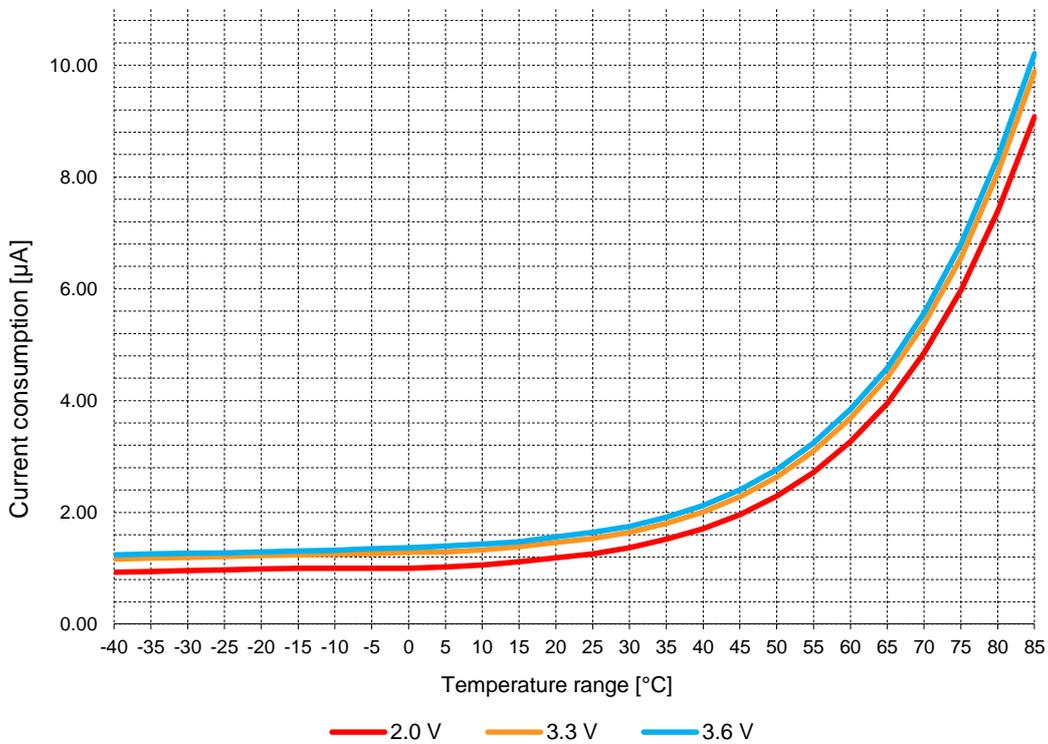
Figure 4: Current consumption during Idle state
