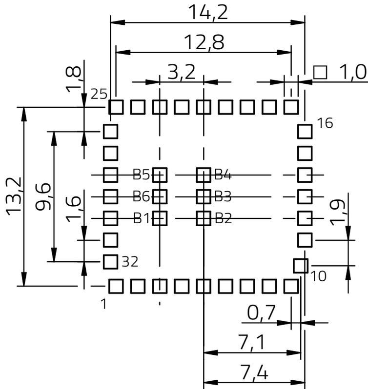
Figure 45: Footprint and dimensions [mm]
