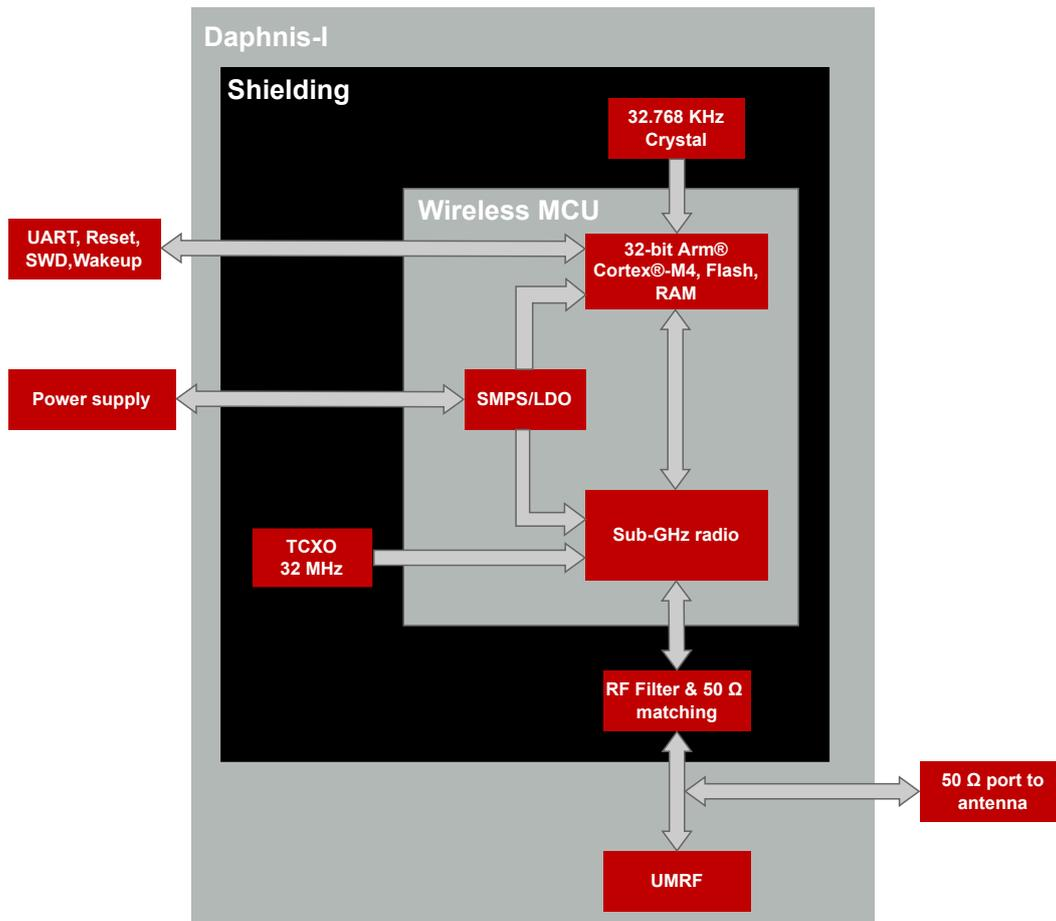
Figure 2: Block diagram
