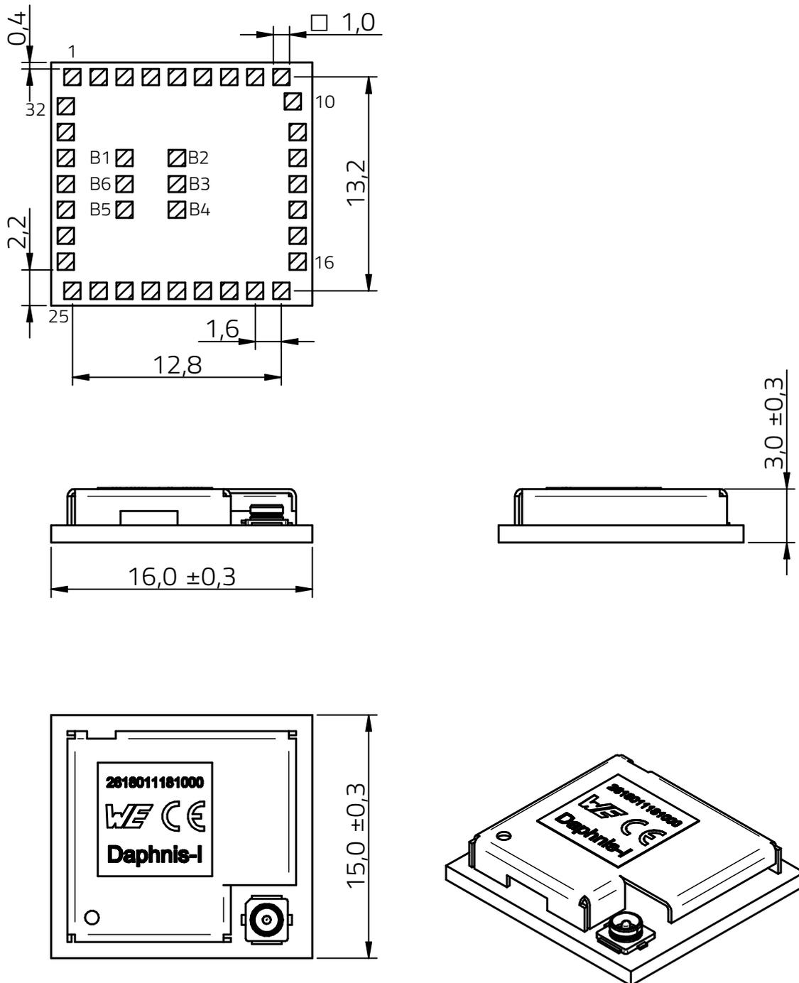
Figure 44: Module dimensions [mm]
