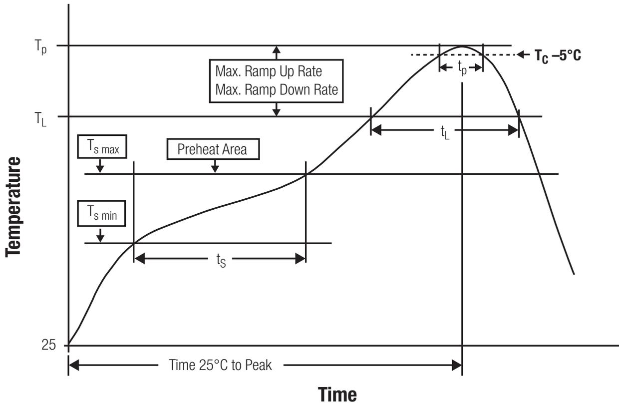
Figure 43: Reflow soldering profile
