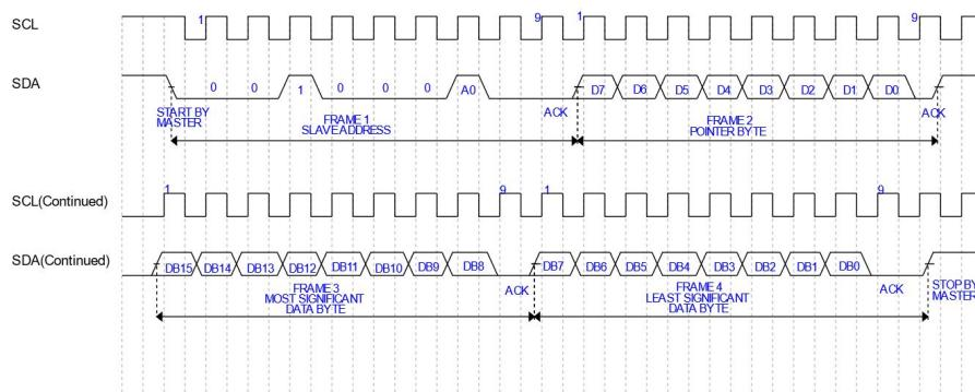
**Figure 7. I<sup>2</sup>C Write**
