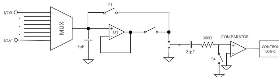
**Figure 6. ADC Input Structure**
