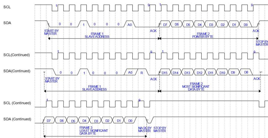
**Figure 10. I<sup>2</sup>C Block Read**
