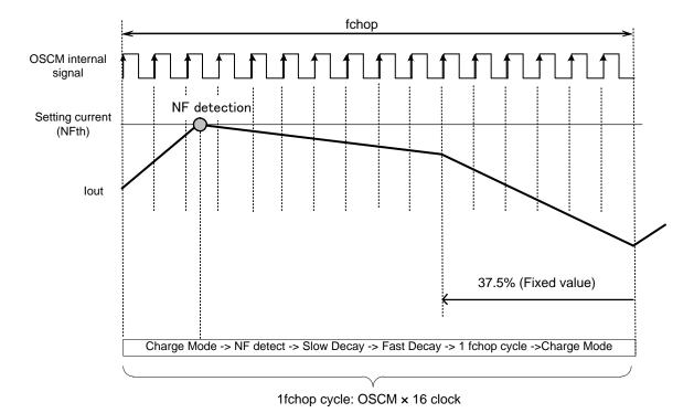
Note: The blanking time(AtBLK) is also set to prevent an incorrect operation in the NF detection (the motor current reaches the set current value (NFth)).
