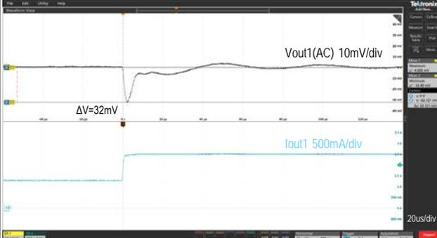
Step Load Transient Response (Vin=5.0V, Vout1=1.2V, Iout1=2.5 to 1.25A)
