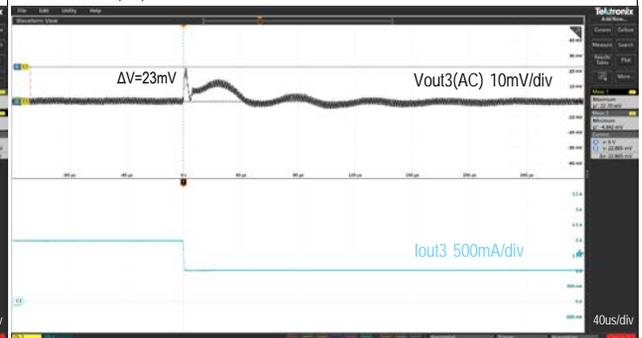
Step Load Transient Response (Vin=5.0V, Vout4=2.5V, Iout4=0.75 to 1.5A)
