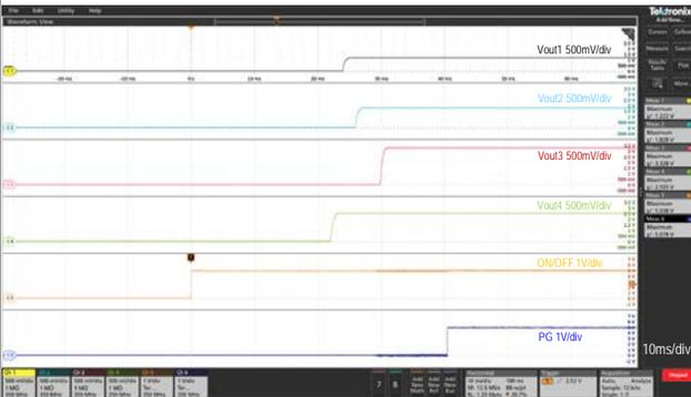
ON/OFF Enable Delay (Vin=5.0V, All Iout=max.)
