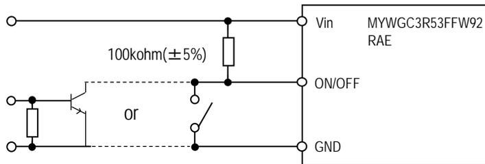
It is strongly recommended that the ON/OFF terminal should be used when turning on/off this product. The characteristics of the ON/OFF function may be affected by turning on/off input voltage. Please check product operation on your application with turning on/off input voltage.
