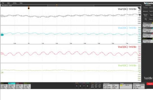
Output Ripple and Noise (Vin=5.0V, All Iout=no load)
