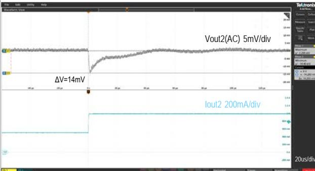
Step Load Transient Response (Vin=5.0V, Vout2=1.8V, Iout2=1.0 to 0.5A)
