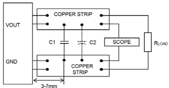
C1= Cout conditions (described in the test circuit for each Vout)
