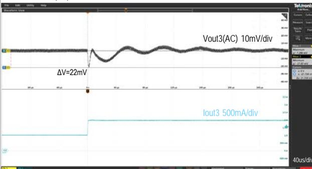
Step Load Transient Response (Vin=5.0V, Vout3=3.3V, Iout3=2.0 to 1.0A)
