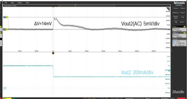
Step Load Transient Response (Vin=5.0V, Vout3=3.3V, Iout3=1.0 to 2.0A)
