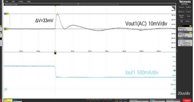
Step Load Transient Response (Vin=5.0V, Vout2=1.8V, Iout2=0.5 to 1.0A)
