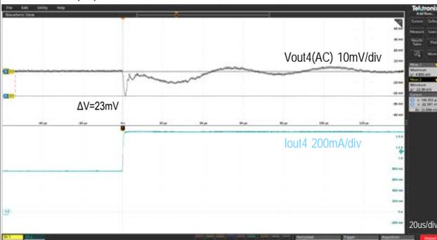
Step Load Transient Response (Vin=5.0V, Vout4=2.5V, Iout4=1.5 to 0.75A)
