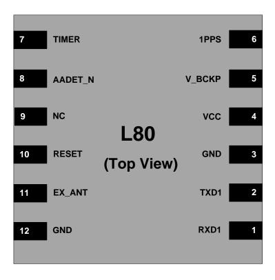
Figure 2: Pin Assignment
