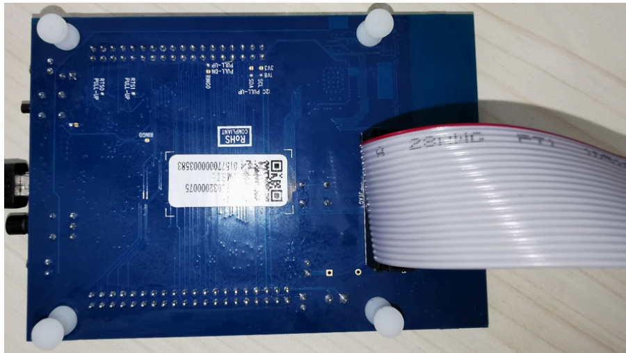
Figure 45. JTAG Connector Detail
