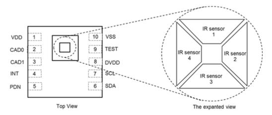
Figure 6.1. IR Sensor's Configurations
