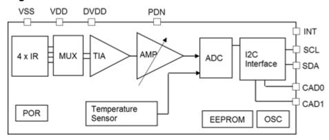
Figure 4.1 AK9750 Block Diagram
