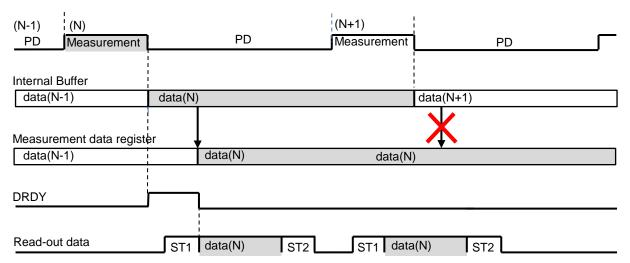
Figure 11.7. Read-out data within a measurement period
