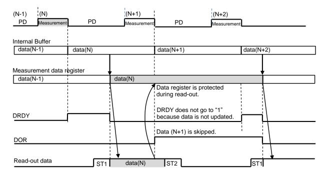
Figure 11.9. The data read cannot be completed until the beginning of the next measurement.
