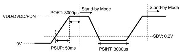
Figure 9.1. Power Supply Conditions
