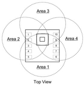
Figure 6.2. IR Sensor's Observable Area
