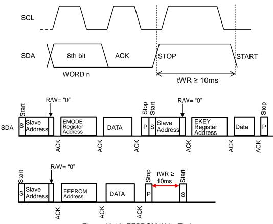
Figure 12.10. EEPROM Write Timing
