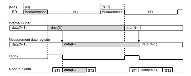
Figure 11.6. Normal Read-out Procedure
