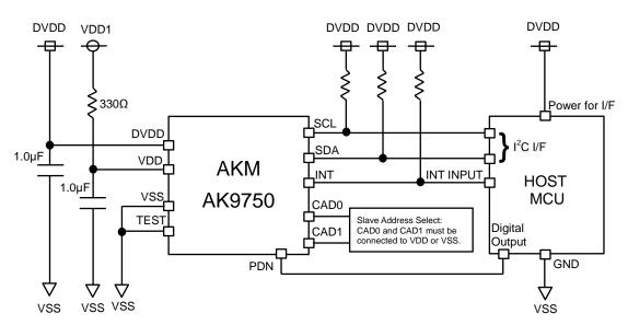
Figure 21.1. Recommended External Circuits
