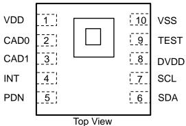
Figure 5.1 Pin Configurations
