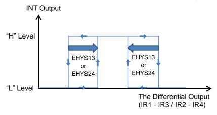
Figure 14.1. Hysteresis setting for threshold levels.
