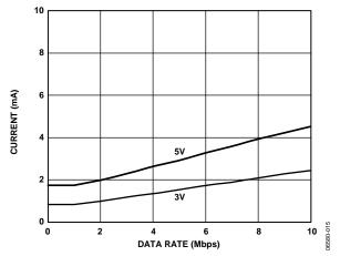
Figure 15. Typical ADuM1412 V<sub>DD1</sub> or V<sub>DD2</sub> Supply Current vs. Data Rate for 5 V and 3 V Operation
