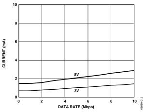
Figure 12. Typical ADuM1410 V<sub>DD2</sub> Supply Current vs. Data Rate for 5 V and 3 V Operation
