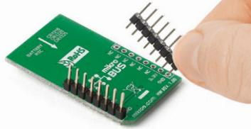
Turn the board upside down so that the bottom side is facing you upwards. Place shorter pins of the header into the appropriate soldering pads.
