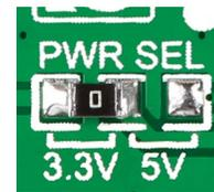
RTC6 click features an SMD jumper (zero ohm resistor) that let's you switch between a 3.3V or a 5V power supply.
