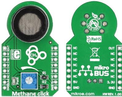
Methane click™ is a simple solution for adding a high sensitivity methane (CH<sub>4</sub>) sensor to your design. It's suitable for designing gas leakage equipment. The board features an MQ-4 sensor, a calibration potentiometer, a mikroBUS™ host socket, two jumpers and a power indicator LED. Methane click™ communicates with the target board through mikroBUS™ AN (OUT) line. Methane click™ is designed to use a 5V power supply only.
