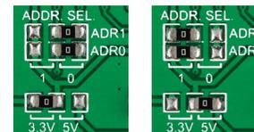
*IrThermo 2 click* has two sets of jumpers. ADDR. SEL. for specifying the I<sup>2</sup>C address, and a jumper for switching between 3.3V and 5V power supplies.
