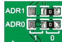
The HDC100 sensor acts as a slave on the I<sup>2</sup>C interface. Two jumpers (zero-ohm resistors)
