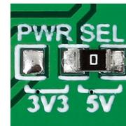
The board features a PWR SEL jumper which is used to determine whether 5V or 3.3V power supply is used.
