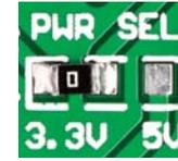
On-board **PWR SEL** zero-ohm resistor (SMD jumper) is used to determine whether 5V or 3.3V power supply is used. This resistor is provided in 3.3V position by default. In order to use DIGIPOT click with 5V development system, it is necessary to resolder this jumper to 5V position.
