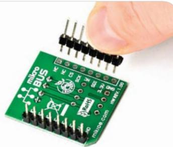
Turn the board upside down, so that bottom side is facing you upwards. Place shorter parts of the header pins in the both soldering pad locations.
