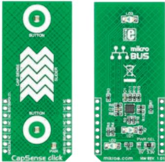
CapSense click™ is an accessory board in **mikroBUS™** form factor. It's a compact and easy solution for adding capacitive sensing elements to your design. It features **CY8C201A0** capacitive controller and capacitive sensing elements. CapSense click™ communicates with the target board microcontroller via **mikroBUS™** I2C (SDA, SCL), AN and RST lines. The board is designed to use 3.3 V or 5 V power supply. LED diode (GREEN) indicates the presence of power supply.
