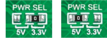
There is one zero-ohm SMD jumper **J1** used to select whether 3.3 V or 5 V power supply is used. Jumper **J1** is soldered in 3.3 V position by default.
