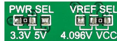
PWR SEL is used to determine whether 5V or 3.3V power supply is used, and VREF SEL to select either VCC or 4.096 V as the voltage reference.
