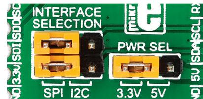
There are two jumpers for SPI/I<sup>2</sup>C selection and one used to select whether 3.3V or 5V power supply will be used.
