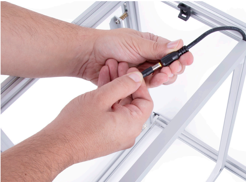
Figure 6: Connecting 12V power plug to the LED connector
