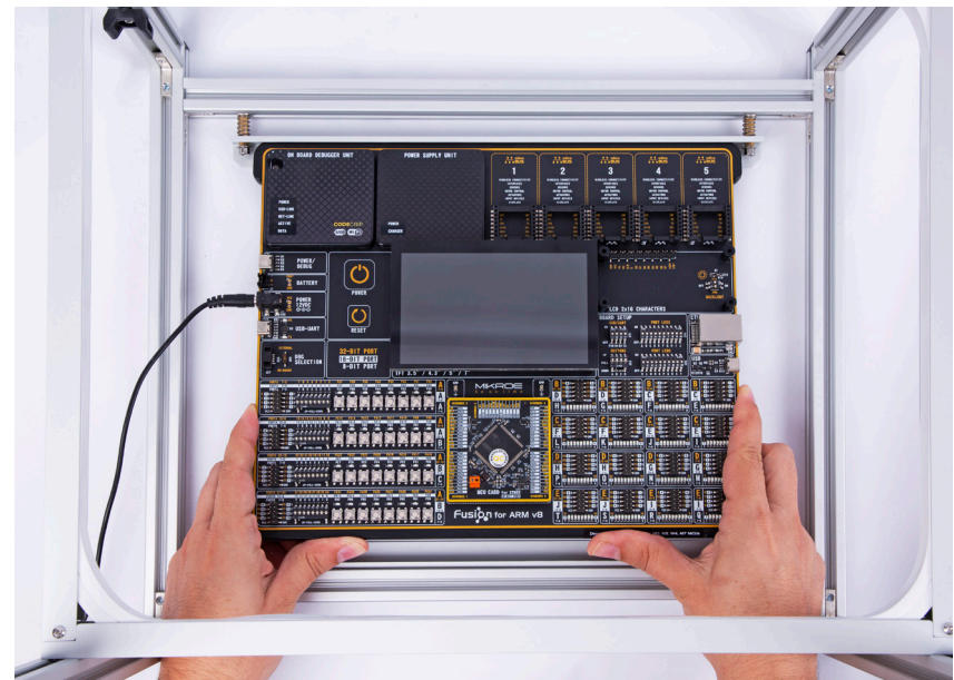
Figure 5: Placing development board into the metal base
