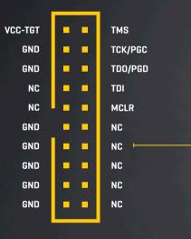
The CODEGRIP device is equipped with the target MCU connector, which contains ICSP/EJTAG and power supply pins. This connector is used to interface the CODEGRIP device with the target MCU, allowing it to perform programming and debugging operations, to provide the power supply for the target MCU, and to be used as the power input when the CODEGRIP device is powered from the connected development board.
