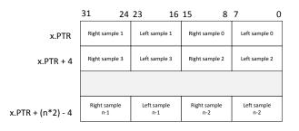
*Figure 27: Memory mapping for 8 bit stereo. CONFIG.SWIDTH = 8Bit, CONFIG.CHANNELS = Stereo.*
