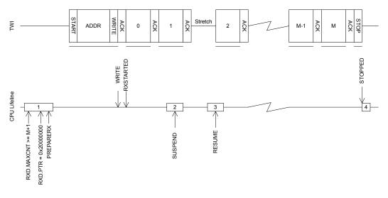
Figure 101: The TWI slave responding to a write command
