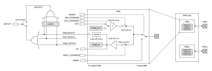
Figure 16: GPIO port and the GPIO pin details
