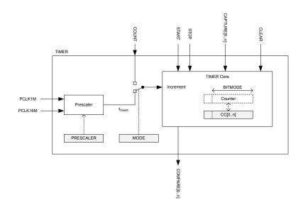
Figure 88: Block schematic for timer/counter
