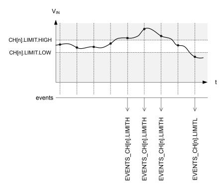
Figure 70: Example of limits monitoring on channel 'n'
