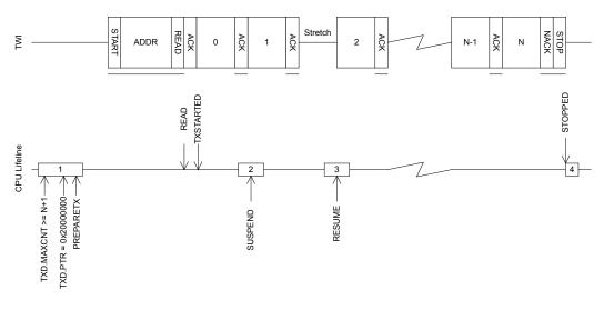
Figure 100: The TWI slave responding to a read command
