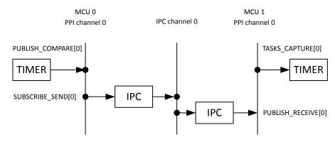
Figure 21: Example of PPI and IPC connections
