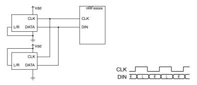
Figure 39: Example of two PDM microphones
