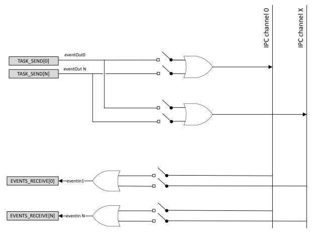
Figure 20: IPC registers SEND\_CNF and RECEIVE\_CNF
