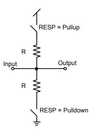
*Figure 68: Resistor ladder for positive input (negative input is equivalent, using RESN instead of RESP)*
