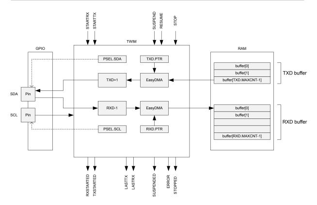
Figure 89: TWI master with EasyDMA
