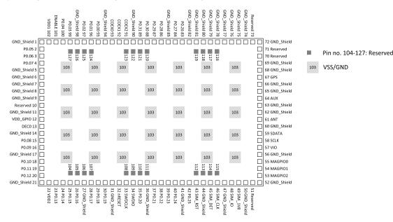
Figure 113: LGA pin assignments, top view
