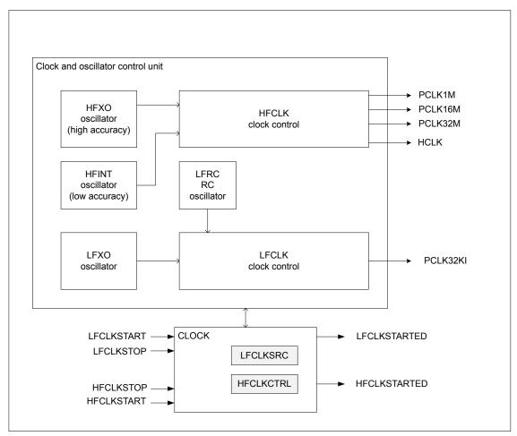
Figure 11: Clock and oscillator setup
