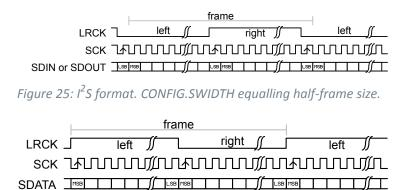
Figure 26: Aligned format. CONFIG.SWIDTH equalling half-frame size.
