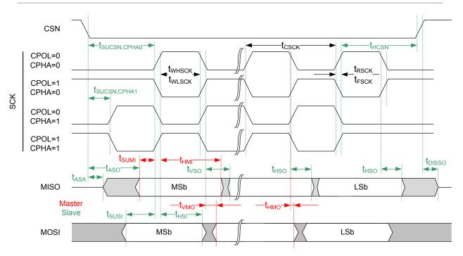
Figure 78: Common SPIM and SPIS timing diagram
