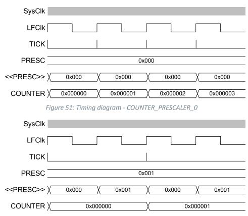
Figure 52: Timing diagram - COUNTER\_PRESCALER\_1
