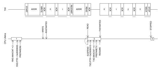
*Figure 102: A repeated start sequence, where the TWI master writes two bytes followed by reading four bytes from the slave*
