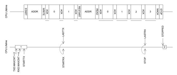
*Figure 93: A repeated start sequence, where the TWI master writes two bytes followed by reading 4 bytes from the slave*
