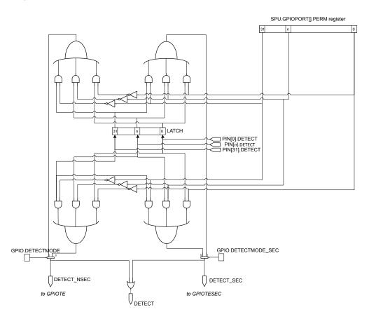
Figure 18: Principle of direct pin access
