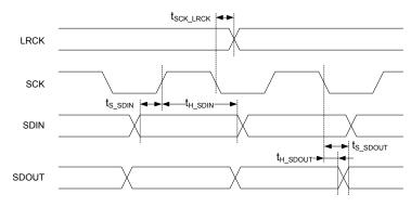
Figure 33: I2S timing diagram
