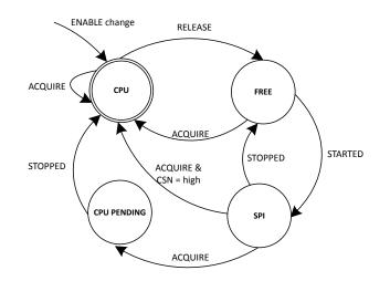
Figure 76: SPI semaphore FSM
