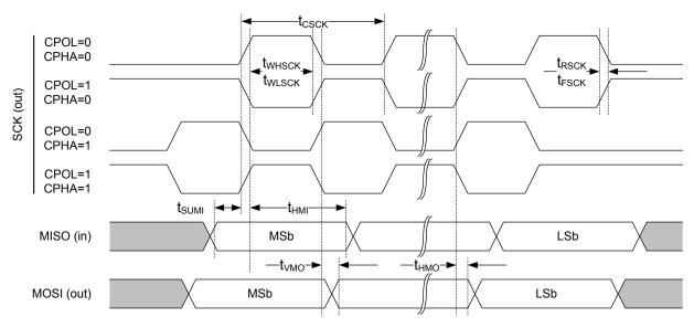
Figure 73: SPIM timing diagram
