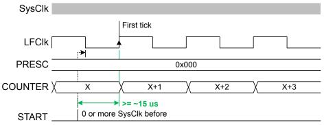
Figure 62: Timing diagram - JITTER\_START-
