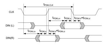
Figure 40: PDM timing diagram
