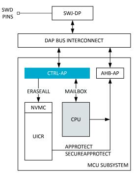
Figure 111: Control access port details
