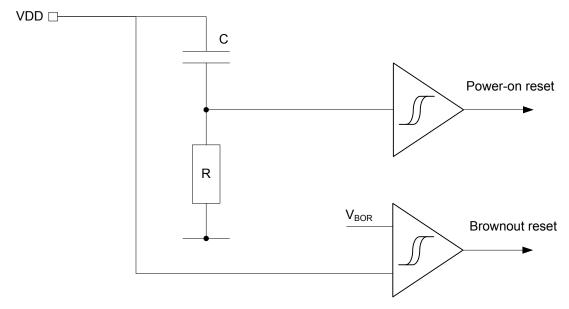
Figure 10: Power supply supervisor
