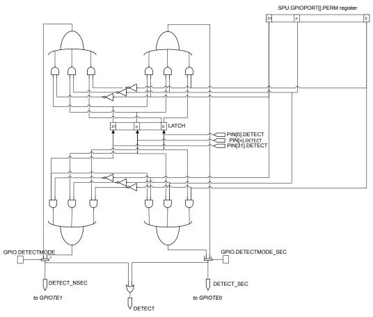
Figure 85: Principle of direct pin access
