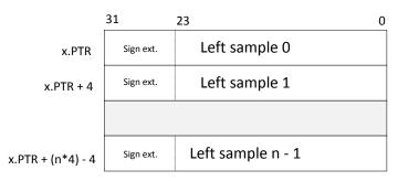
Figure 32: Memory mapping for 24 bit mono, left channel only. CONFIG.SWIDTH = 24Bit, CONFIG.CHANNELS = Left.
