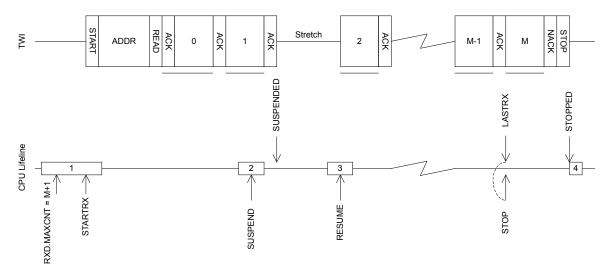
Figure 92: The TWI master reading data from a slave
