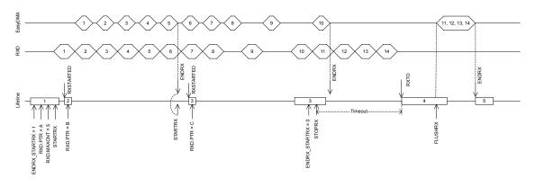
Figure 107: UARTE reception with forced stop via STOPRX
