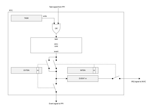
Figure 53: Tasks, events and interrupts in the RTC
