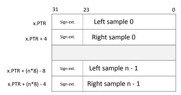
Figure 31: Memory mapping for 24 bit stereo. CONFIG.SWIDTH = 24Bit, CONFIG.CHANNELS = Stereo.
