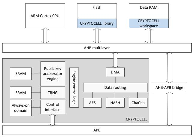
Figure 12: Block diagram for CRYPTOCELL
