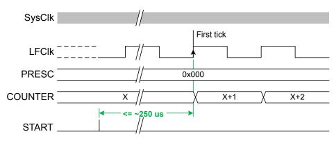
Figure 63: Timing diagram - JITTER\_START+
