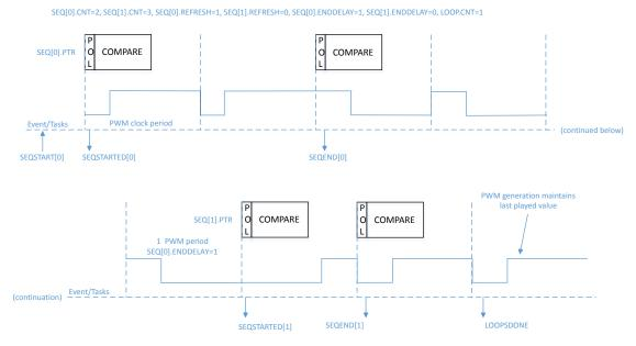
Figure 46: Example using two sequences
