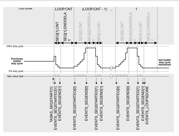
Figure 49: Complex sequence (LOOP.CNT>0) starting with SEQ[1]
