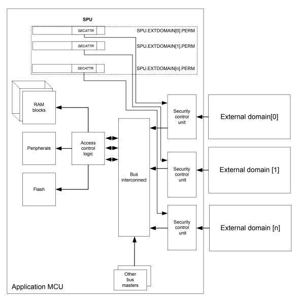
Figure 87: Access control from external domains
