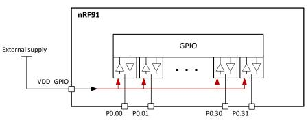
Figure 9: GPIO supply input (VDD\_GPIO)
