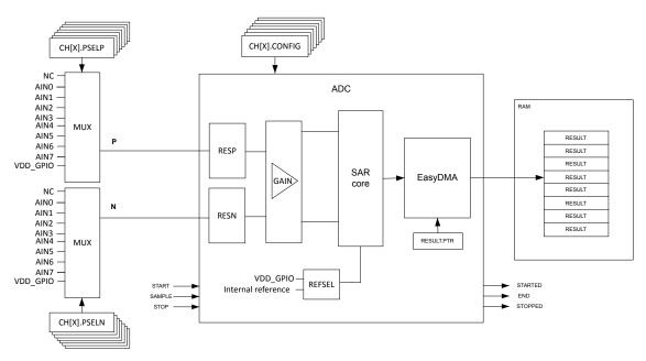
Figure 64: Simplified ADC block diagram
