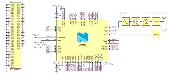
Figure 115: Schematic SIxA with antenna details
